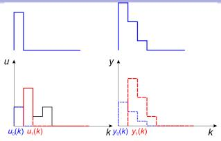
Consider a signal  $\tilde{u}_i(k)$  equal to u(j) at k = j, and 0 elsewhere; just a shifted and scaled unit impulse:
