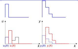
Consider a signal  $\tilde{u}_j(k)$  equal to u(j) at k = j, and 0 elsewhere; just a shifted and scaled unit impulse:
