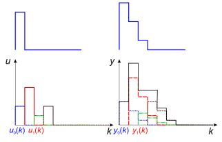
Now, u(k) is the superposition of all signals  $\tilde{u}_j$ , so due to linearity:
