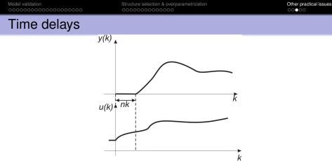
Read the delay on the graph. Set *nk* appropriately in Matlab, or otherwise add *nk* leading zeros to the polynomial  $B(q^{-1})$  in the model:
