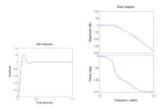
The model represents the system behavior in graph form, such as *step response* or *frequency response* (Bode diagram). The next lectures will deal with this type of model (step & impulse responses).
