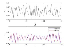
Our goal of simulating the system output is achieved (for inputs that are "well represented" by the experimental input chosen).
