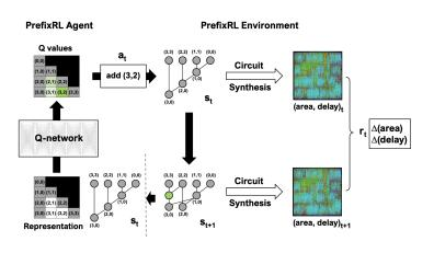
Learn optimal placement of parallel prefix circuits such as adders while optimising for area, delay and power.
