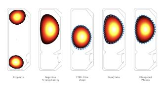
Various plasma shapes obtained by the learned controller, including a novel "droplets" configuration.
