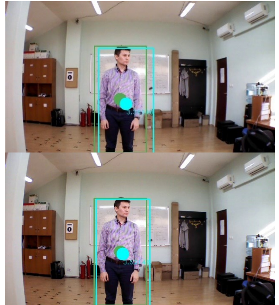
Fig. 2. Measured and filtered box in two subsequent frames
