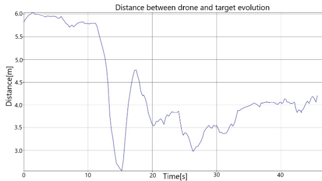
Fig. 5. Evolution of distance between drone and target during a control experiment
