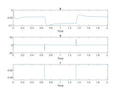
Similarly to the open-loop case, the system has order 2 and the disturbance is colored (does not obey the ARX model structure).
