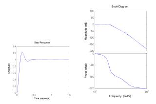
The model represents the system behavior in graph form, such as *step response* or *frequency response* (Bode diagram).
