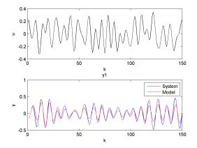
Our goal of simulating the system output is reasonably achieved (for inputs that are "well represented" by the experimental input chosen).
