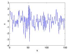
Recall zero-mean white noise: mean 0, different steps uncorrelated. In the figure, values were independently drawn from a zero-mean Gaussian distribution.
