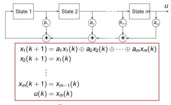
$x(k) = [x_1(k), \dots, x_m(k)]^{\top}$  compactly denotes the state vector of m variables (bits)
