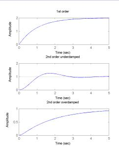
Even when it is overdamped or critically-damped, at t=0 a 2nd order system response will have a derivative of 0: it will be tangent to the time axis. In contrast, the tangent slope is K/T for 1st order systems.
