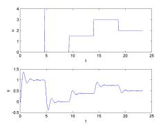
Note again the measurement noise. Also, while the experiment has zero initial condition ( $u_0 = y_0 = 0$ ), the steps still have nonstandard values (different from 1).
