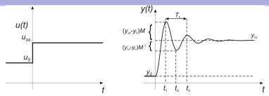
Similar to 1st order case: new input  $u(t) = u_0 + (u_{ss} - u_0)u_s(t)$ , so the new output is again just a shifted and scaled version of the ideal step response  $y_S(t)$ :  $y(t) = y_0 + (u_{ss} - u_0)y_S(t)$ . Modified algorithm:
