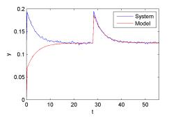
The simulation does not take into account the nonzero initial condition of the system, hence the first part has large differences.
