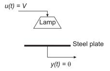
Consider the thermal system in the figure (different from the example above). The input is the voltage V applied to the lamp, the output is the temperature  $\theta$  read by a thermocouple at the back of the steel plate.
