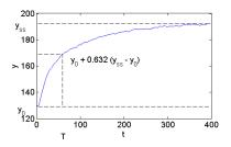
We have  $y_{ss} \approx 192^{\circ}$  C,  $y_0 \approx 129^{\circ}$  C. Also, the input  $u_{ss} = 9$  V and (from the experiment) we know that  $u_0 = 6$  V. Therefore:
