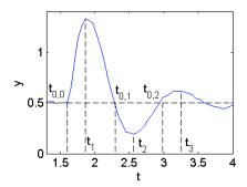
We read  $t_1 \approx 1.92$  and  $t_3 \approx 3.2$ , leading to  $T_0 = 1.28$ . From this,  $\omega_n = \frac{2\pi}{T_0\sqrt{1-\xi^2}} \approx 5.16$ .
