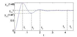
Since the output is noisy, we determine the steady state value by averaging a few last samples in steady-state, namely numbers 90 to 100, between  $t_4$  and  $t_5$ :
