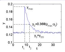
The maximum output value is  $y_{\text{max}} \approx 0.19$ , reached at  $t_1 \approx 8.86$ . Value  $y_0 + 0.368(y_{max} - y_0) \approx 0.15$  is reached at  $t_2 \approx 12.60$ . Therefore:
