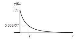
We can estimate the gain by using  $y_{\text{max}} = \frac{K}{T}$ , but in practice this will not be as accurate (e.g. because of noise and the non-ideal impulse signal).
