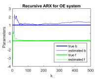
Conclusion: Convergence to the true values is not attained! – due to colored noise (system not in model class)
