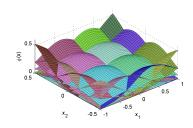
Results with  $6 \times 6$  RBFs, with centers on an equidistant grid and width equal to the distance between two centers:
