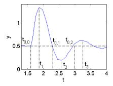
We read  $t_1 \approx 1.92$  and  $t_3 \approx 3.2$ , leading to  $T_0 = 1.28$ . From this,  $\omega_n = \frac{2\pi}{T_0\sqrt{1-\xi^2}} \approx 5.16.$
