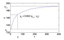
The nonparametric model is the graph. We use it to estimate a transfer function model.
