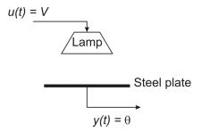
Consider the thermal system in the figure (different from the example above). The input is the voltage V applied to the lamp, the output is the temperature  $\theta$  read by a thermocouple at the back of the steel plate.
