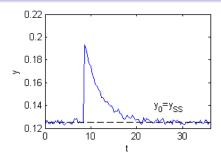
We use the graph (nonparametric model) to estimate a transfer function (parametric model). We have  $u_0 = u_{ss} = 0.5$ .
