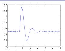
We use the graph (nonparametric model) to estimate a transfer function (parametric model). We have  $u_0 = u_{ss} = 2$ .
