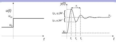
Similar to 1st order case: new input  $u(t) = u_0 + (u_{ss} - u_0)u_s(t)$ , so the new output is again just a shifted and scaled version of the ideal step response  $y_S(t)$ :  $y(t) = y_0 + (u_{ss} - u_0)y_S(t)$ . Modified algorithm:
