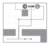
**Figure 8.** A solution obtained with *team Q-learning*. Agent 1 travels along the thick gray line, and agent 2 along the thin black line. Dots mark the states where the agents stand still; the size of each dot is proportional with the time spent standing still in that cell.
