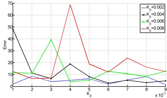
Fig. 9: PID tuning results based on the grid, on the Y axis is the error, on the X axis the values for  $K_d$ , and the different colored lines correspond to different values of  $K_p$ .
