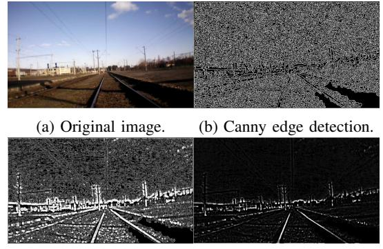
Fig. 4: Comparison of edge detection methods.
