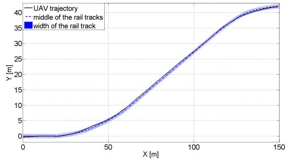
Fig. 11: Trajectory of the drone in the simulation, following a rail track with turns.
