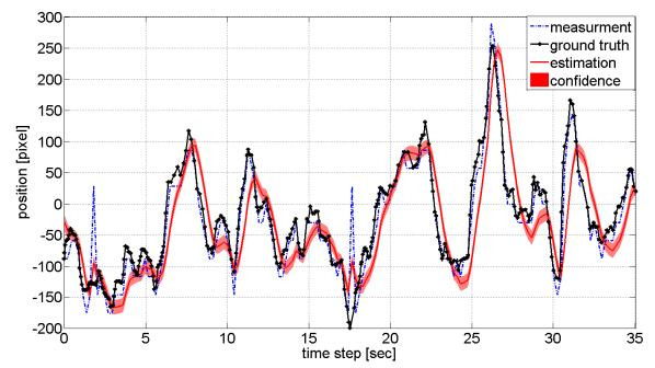
Fig. 5: Detection and KF estimation analysis on frequently used tracks. The dashed (blue) line is the measurement, the dotted (black) line is the ground truth labeled by hand frame by frame, the continuous (red) line is the estimation and the shaded (red) surface is the 95% confidence interval on the estimation.
