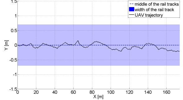
Fig. 10: Trajectory of the drone in the simulation following a straight rail track, where the black line is the trajectory, the blue line is the middle of the track and the blue shade is the width of the track.
