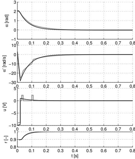
Fig. 3. Controlled trajectory of the DC motor with OPC (gray) and the optimal solution (black), from  $x_0 = [2\pi/3, \pi]^T$ .
